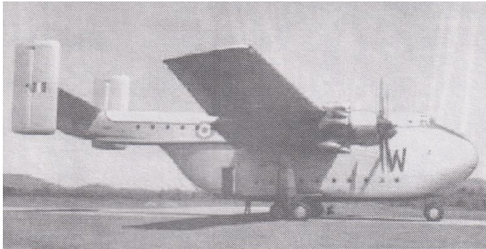
Above - The Beverley Aircraft so designed that parachutists could be carried and jump from the tail and their vehicles/plant machinery carried and dropped by parachutes from the main body, or alternatively all parachutists. Right — Land Rover and trailer on platform having just dropped by parachute
